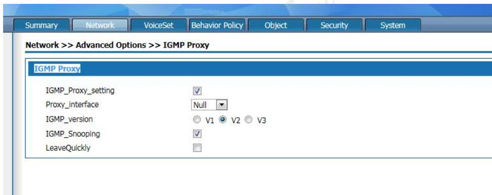
Figure 4-22 IGMP Proxy setting
