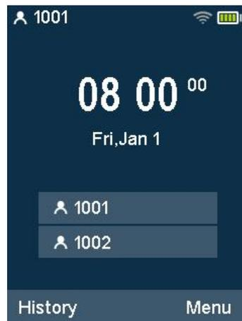
The phone standby interface can display the phone's time, date, phone status (Do Not Disturb, Auto Answer), account registration status, extension number, label, battery level and WIFI icon, and two soft keys at the bottom of the LCD screen (History , Menu) label. For the description of the icons on the standby interface, please refer to the display icon composition.
