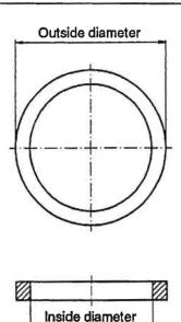
b) Type IBC gasket (for type A and type B flange facings). Type TG gasket (for type C/D flange facings). Type SR gasket (for type E/F flange facings).
